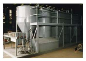
Water treatment systems are typically supplied as modular shop-built systems that are completely assembled, tested, and ready to run. Custom modifications to suit site specific criteria can be easily accommodated. Portable systems suitable for construction sites or temporary requirements are also available. A one GPM pilot plant is offered on a rental basis to test various process methods on site before committing to a full scale system.
